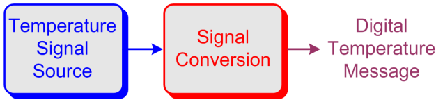
Fig. 3. Flow diagram of a smart temperature sensor.
