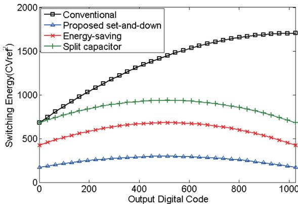
Fig. 3. Switching energy vs. output digital code.
