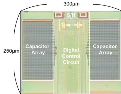
Fig. 5. Die photo of the proposed SAR ADC.
