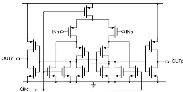
Fig. 4. The schematic of the comparator.
