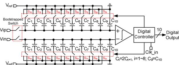
Fig. 1. The proposed SAR ADC.
