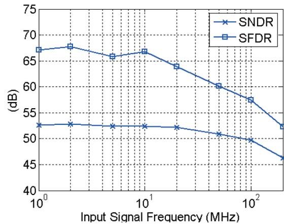
Fig. 6. SFDR and SNDR vs. input frequency at 50 MS/s.
