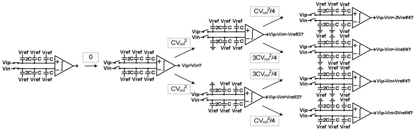
Fig. 2. A 3-bit example of proposed set-and-down switching procedure.
